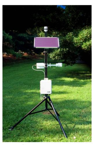
The LP-AWS® is an advanced, portable, Low Power Automated Weather Station built around the OWI-650 Low Power Weather Identifier and Visibility Sensor (LP-WIVIS®). The low power requirements of the OWI-650 make it well suited for portable battery and solar powered applications. The system has been designed from the ground up for fast setup anywhere.
