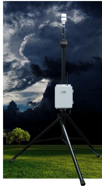
The OWI-650-DS Low Power Weather Identifier and Visibility Sensor (LP-WIVIS) is a plug-in option to the HazMet100 system. The LP-WIVIS adds visibility, precipitation intensity and precipitation type discrimination (present weather) to the system. A solar powered option allowing for long term deployment is also available.
