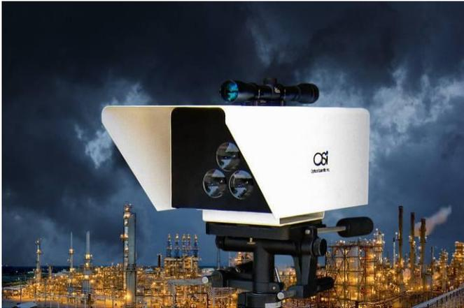
**OSi's Optical Wind and Visibility sensor (OWV)** is a breakthrough in measuring turbulence, large body air / wind movement and atmospheric visibility over a long path (50 to 300 meters or more) – all in a single, low cost sensor. The sensor operates on a combination of long path optical extinction and optical scintillation. All the electronics are housed in the OWV with a folded path being established by placing a corner cube reflector down-range at the desired distance.
