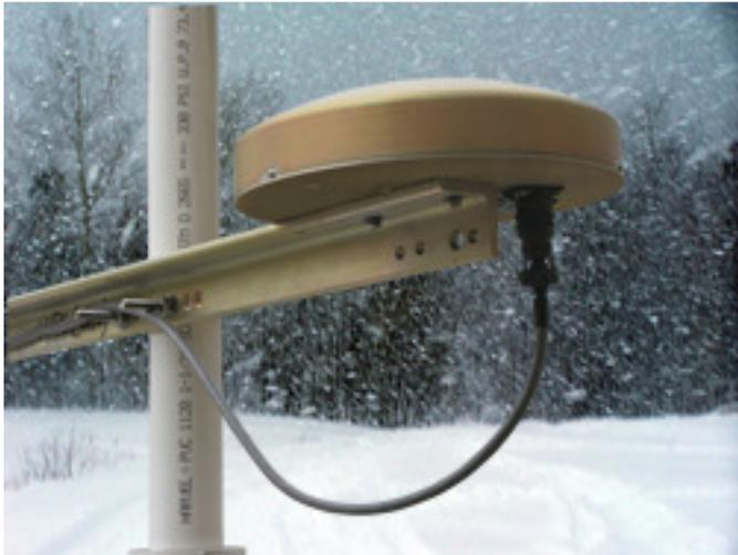
**HIP -100 Hail and Ice Pellet Sensor** is an acoustic sensor developed as an add-on option to OSi's OWI-430 series Weather Sensor, giving an even greater range of weather data collection.
